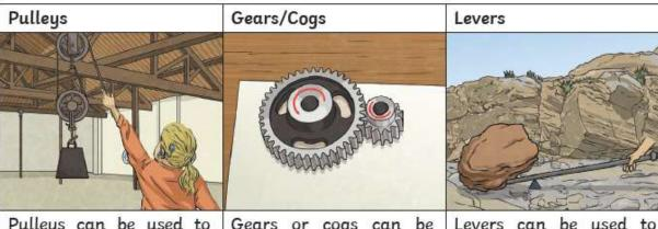
Pulleys can be used to make a small force lift a heavier load. The more wheels in a pulley, the less force is needed to lift a weight.
